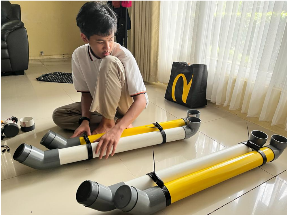
Author, when assembling the SPAT Boat's hull
