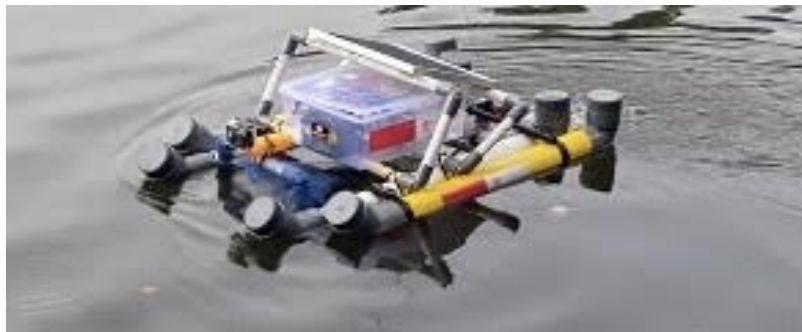
Picture 4.1.2 buoyancy testing
