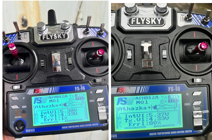
Picture 4.1.4 Change in error when distance is increasing
