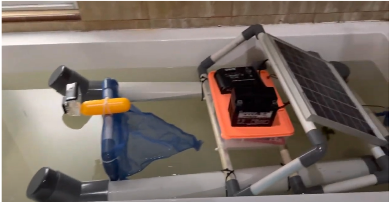
SPAT Boat when doing its initial buoyancy test Link youtube video : https://youtu.be/dN7RCXB38mY
